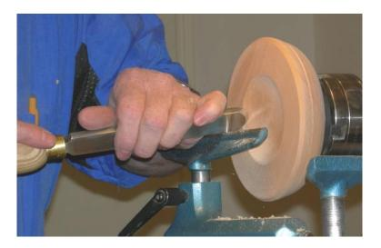
The base was then put back on again, clamping on the inside of where the spindle will fit. Remove the area previously used ot hold the workpiece, so that it's not obvious how it was held.
