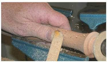
The second bevel can give you more clearance when turning the fiddly bits out.
